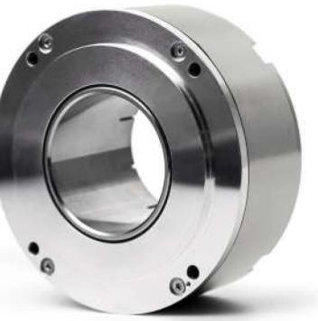
A110H is a photoelectric hollow shaft angle encoder that produces up to 1.800.000 output pulses per revolution and has the accuracy of  $\pm 5$  arc. sec.
