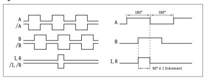
The logical condition of signals A and B is not defined in reference to the index signal I or the reference signal R. It can deviate from the signal form.
